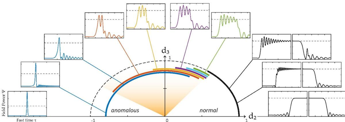
**Localised dissipative structures** that exist in Kerr cavities across the GVD phase space.  $d_2$ : group-velocity (second-order) dispersion,  $d_3$ : third-order dispersion. Clockwise from left: dissipative solitons, dissipative solitons with dispersive tail, zero-dispersion solitons of period -2, 3, 4+, switching wave fronts with dispersive wave tail, switching waves.
